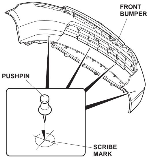
4. While wearing eye protection, drill a 10 mm hole through each marked location from the outside of the bumper. First drill with a 3 mm bit, and finish with a 10 mm bit. Remove any burrs from the edges of the holes with a file.
