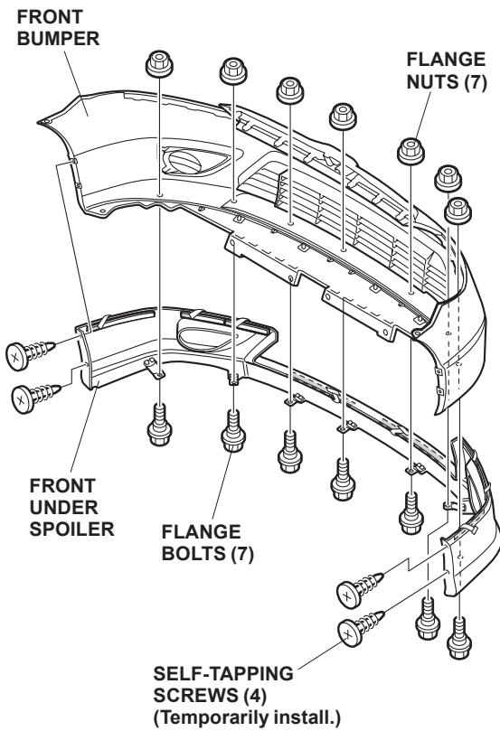
9. Position the front under spoiler on the front bumper, and temporarily install the four self-tapping screws.
