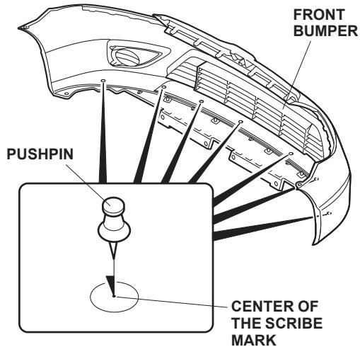
4. Using a drill, drill a 10 mm hole through each marked location from the front of the bumper. First drill with a 3 mm bit, and finish with a 10 mm bit. Remove any burrs from the edges of the holes with a file.
