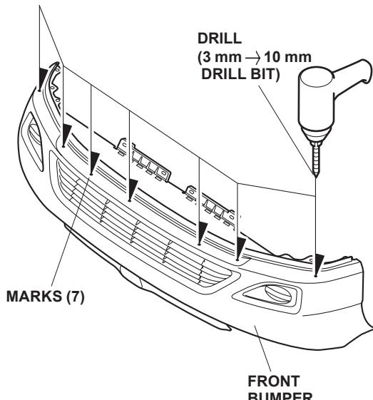
5. Using a drill, drill a 3 mm hole through four dimpled areas of the front bumper on both sides. Remove any burrs from the edges of the holes with a file.
