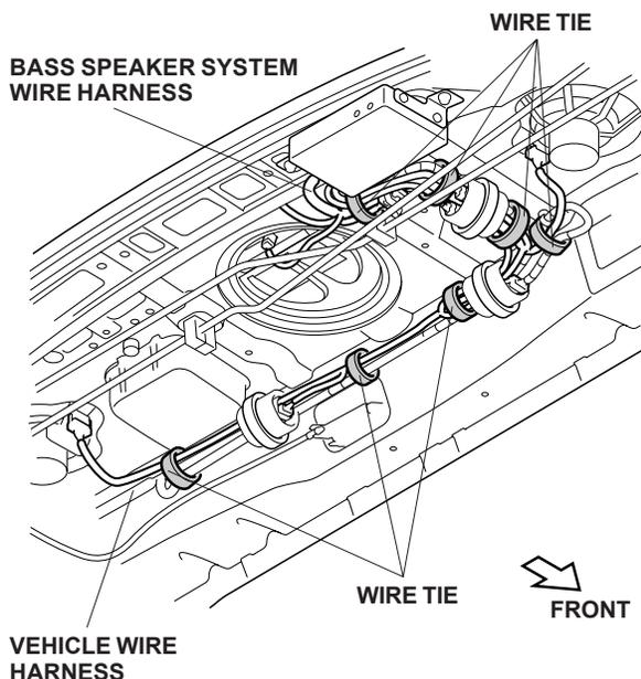
29. Check that all wire harnesses are routed properly and all connectors are plugged in.
