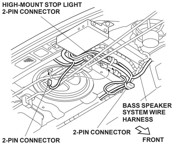
23. Route the high-mount stop light 2-pin connector over the trunk spring, then plug it into the 2-pin connector taped to the bass speaker system wire harness.
