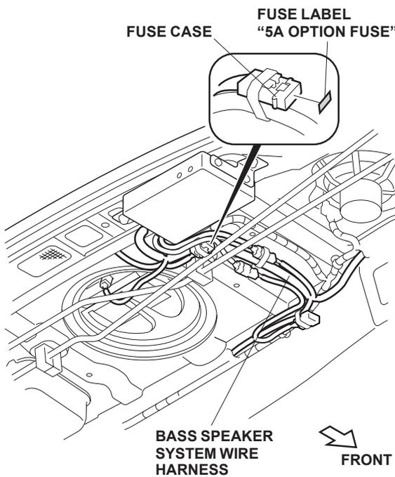
25. Unplug the vehicle 2-pin connector from the vehicle right and left speakers, then plug them into the 2-pin connectors taped on the long branch of the bass speaker system wire harness.
