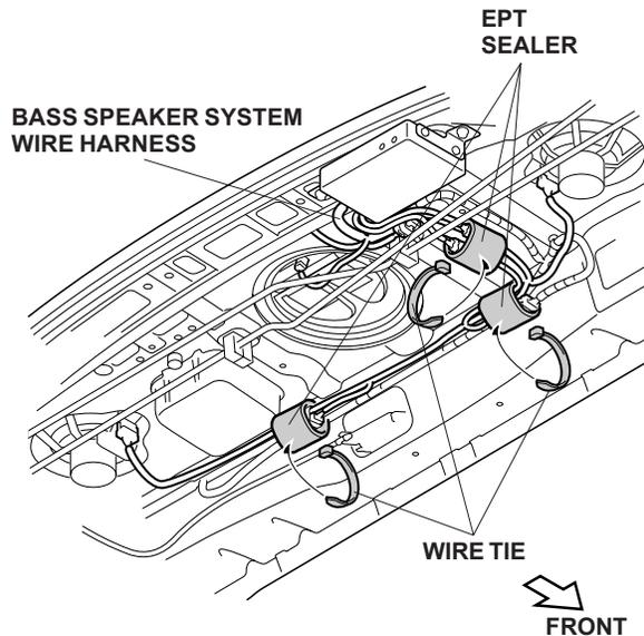
28. Using seven wire ties, secure the bass speaker system wire harness to the vehicle harness in the areas shown.
