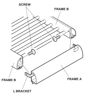
6. Attach the remaining frame A to frame B the same way.
