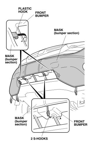
13. Attach four S-hooks to the bottom inside edge of the front bumper and inner fender as shown.
