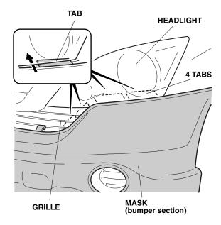
11. Attach the four plastic hooks to the top inside edge of the front bumper.
