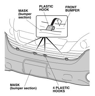
12. Attach the two plastic hooks and two S-hooks to the bottom inside edge of the front bumper.
