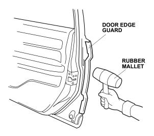
7. Repeat steps 3 through 6 to install the left front door edge guard.
