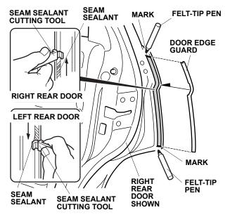
9. Apply touch-up paint to the cut seam sealant area, and let it dry.
