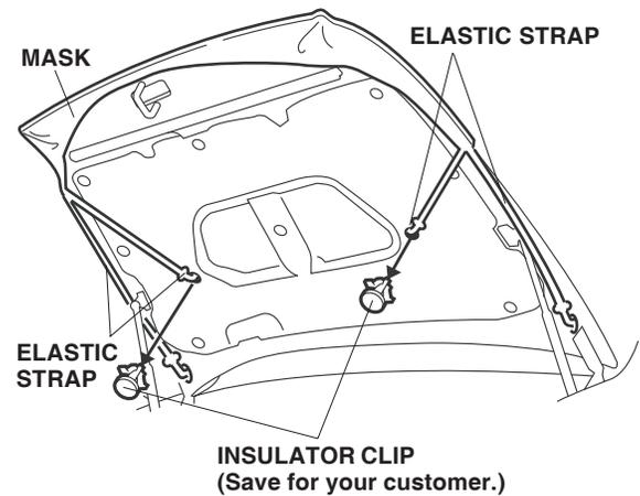
2. Fit the corners of the mask around the hood, and adjust the mask so it fits smoothly over the edges. Secure the mask by hooking the four elastic straps into the holes in the hood.
