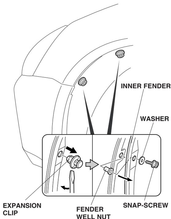
5. Pull out on the inner fender, and press two fenderwell nuts into the holes in the fender flange.
