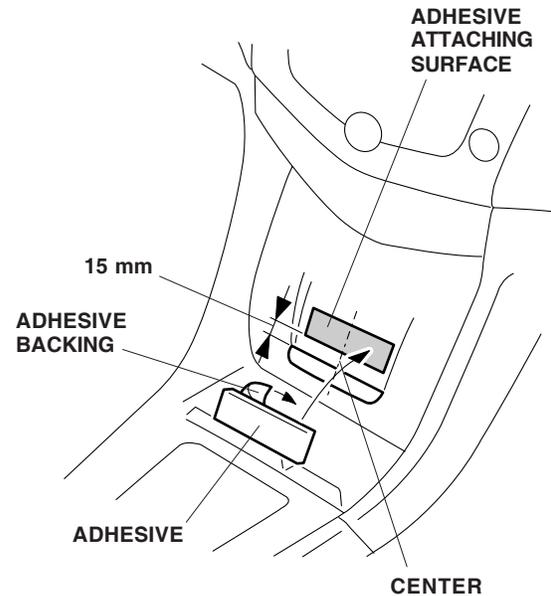
4. Remove and discard the adhesive backing from the adhesive, then attach the adhesive to the center pocket lid as shown.
