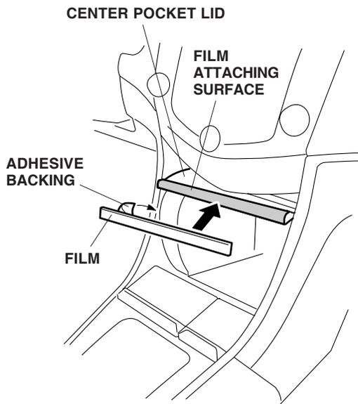
2. Remove the adhesive backing from the film, and attach it to the center pocket lid aligning the lower edge of the film with the lower end of the curved surface of the center pocket lid.
