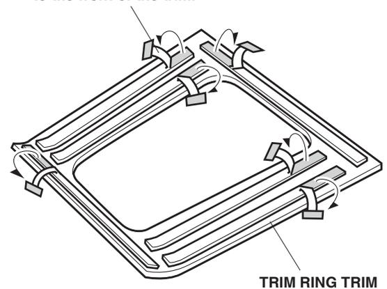
12. Position the trim on the existing trim. While applying light pressure on the trim, carefully remove the adhesive backings.
