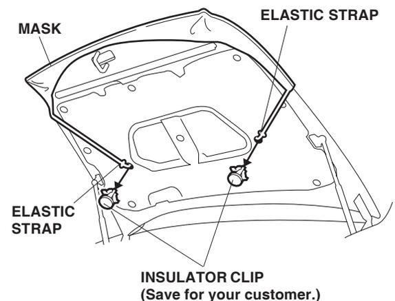
2. Fit the corners of the mask around the hood, and adjust the mask so it fits smoothly over the edges. Secure the mask by hooking the two elastic straps into the holes in the hood.
