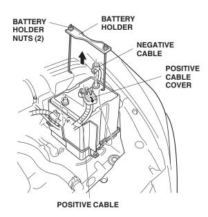
7. Loosen the two battery holder nuts, and remove the battery holder.
