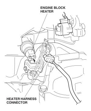
16. Secure the heater harness to the vehicle bracket with one wire tie with clip at the white mark, and secure the heater harness to the vehicle connector with one wire tie at the other white mark.
