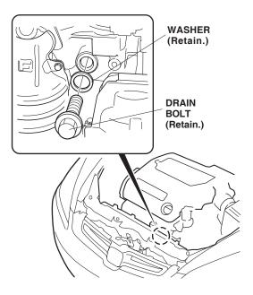
13. Install the engine block heater with the aluminum washer into the hole using a 24 mm socket and a torque wrench. Torque the engine block heater to 60 N·m (44 lb-ft).
