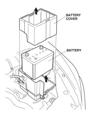
9. Remove the positive (+) cable from the battery box (one clip and one wire tie with clip).
