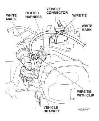
17. Route the heater harness as shown, and secure the heater harness to the fan shroud and vehicle harness with three wire ties. Using a wire tie, secure the white mark point of the heater harness to the fan shroud.
