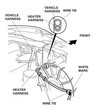
18. Secure the heater harness to the vehicle harness with one wire tie. Do not allow the heater harness to contact the A/C condenser or the radiator.
