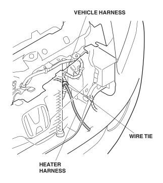
Continue routing the heater harness along the bumper grille opening, and secure the heater harness to the bumper grille with five wire ties.
