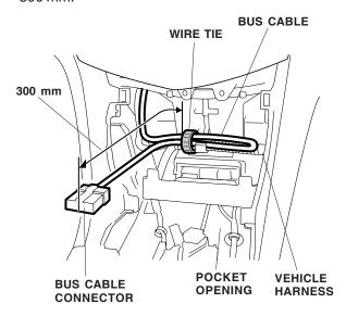
24. Plug the BUS cable connector into the vehicle connector or the player connector. Insert the studs of the left and right player subbrackets and player base-bracket into the holes in the left and right player brackets, then install one 6 mm flange nut on the end of each stud.
