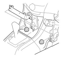
14. Insert the studs of the left and right player subbrackets into the holes in the vehicle frame. While pushing each subbracket upward, install one 6 mm flange nut on the end of each stud.
