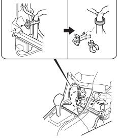
Remove the vehicle clip from the left side of the
