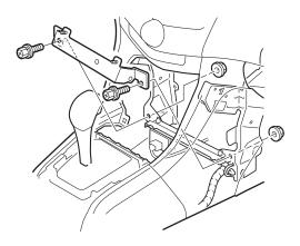
13. Insert the studs of the player base-bracket into the holes in the vehicle frame from the back, then install the two 6 mm flange nuts while holding the bracket firmly against the vehicle frame.
