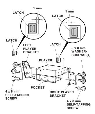
17. Position the left and right player brackets on the player and pocket, and install four 5 x 8 mm washer-screws and two 4 x 8 mm self-tapping screws.
