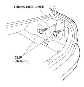
Install the two self-tapping hooks and two screw hooks into the clip holes in the trunk side liner as shown.
