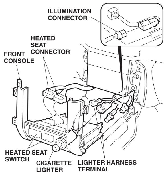
14. Plug the two heated seat connectors into the heated seat switches.
