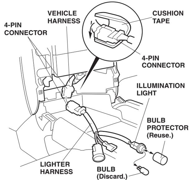
11. Remove the bulb from the illumination light, and reinstall the bulb protector.
