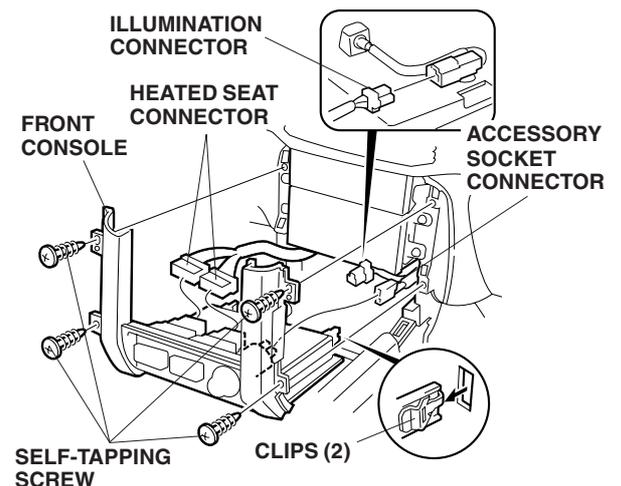
5. Pull out and remove the front console by releasing the two clips, and unplug the accessory socket connector, illumination connector and two heated seat connectors, then remove the front console.
