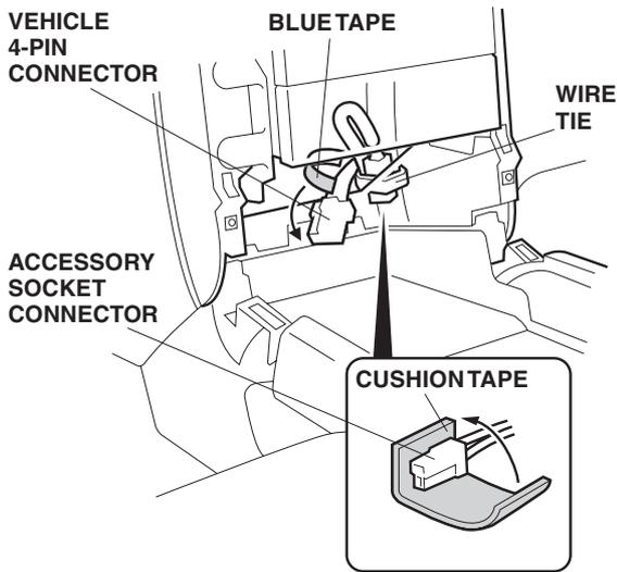
7. Wrap the cushion tape around the accessory socket connector, and secure it to the vehicle harness with one wire tie.
