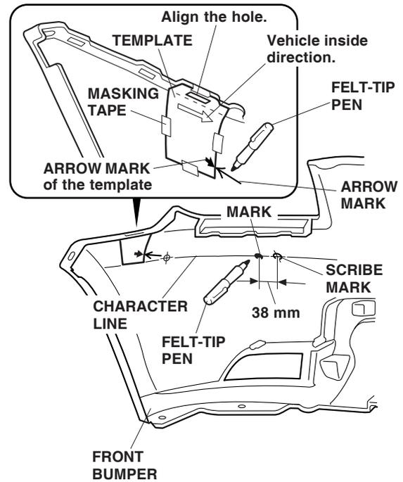
4. Using a felt-tip pen, add the arrow mark to the front bumper against the arrow mark on the template. Drill point is top of arrow.
