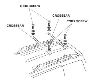
6. *EX model only:* Using a T-25 Torx driver, remove the Torx screws from one end of the roof rack crossbars (front and rear). Remove the end cap. Remove the roof rack end caps from the same side of the vehicle.
