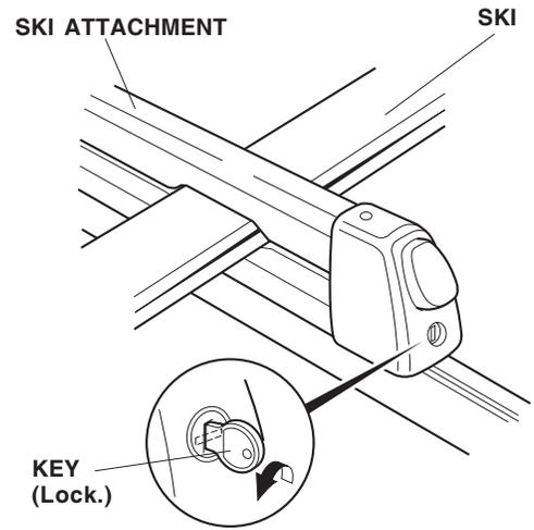
5. With the ski attached, rock the attachment in all directions to make sure it is installed securely. Adjust as necessary.
