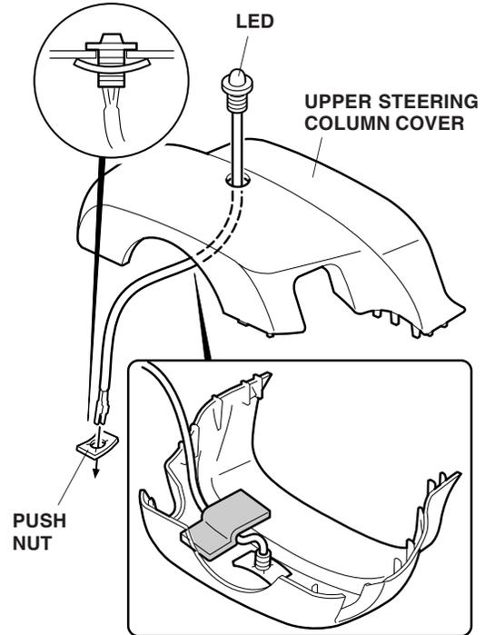
13. Get the 2-pin connector from the kit. Firmly push the LED terminals into the 2-pin connector and lower the lock as shown.
