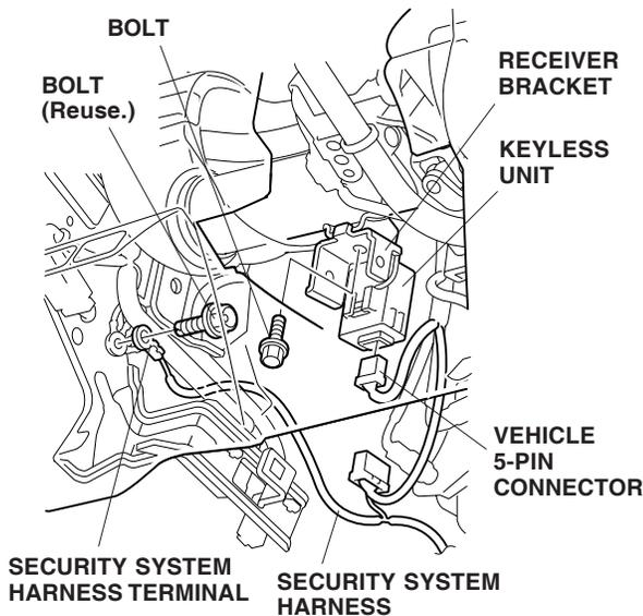
22. Remove the bolt that secures the vehicle ground terminal, and attach the security system harness ground terminal with this bolt.
