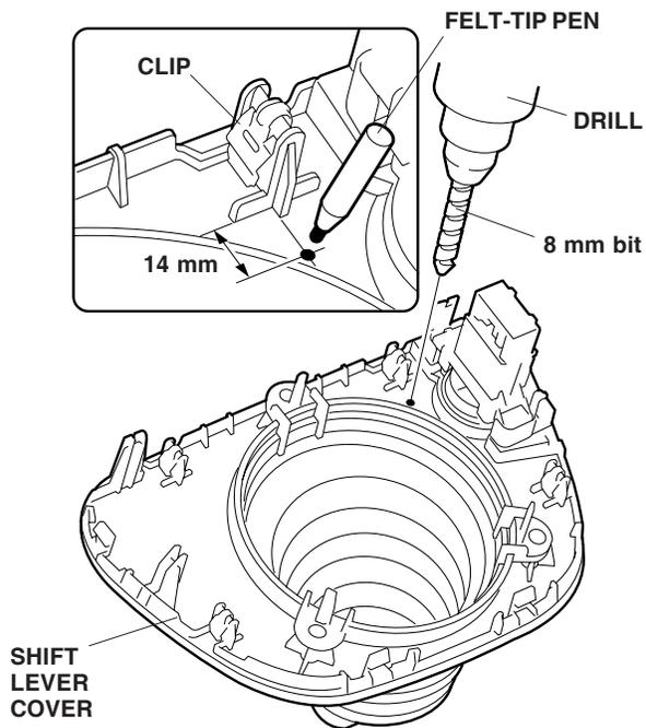
15. While wearing eye protection, lightly center-punch the mark, and drill an 8 mm hole through the center-punched mark. Remove all burrs.
