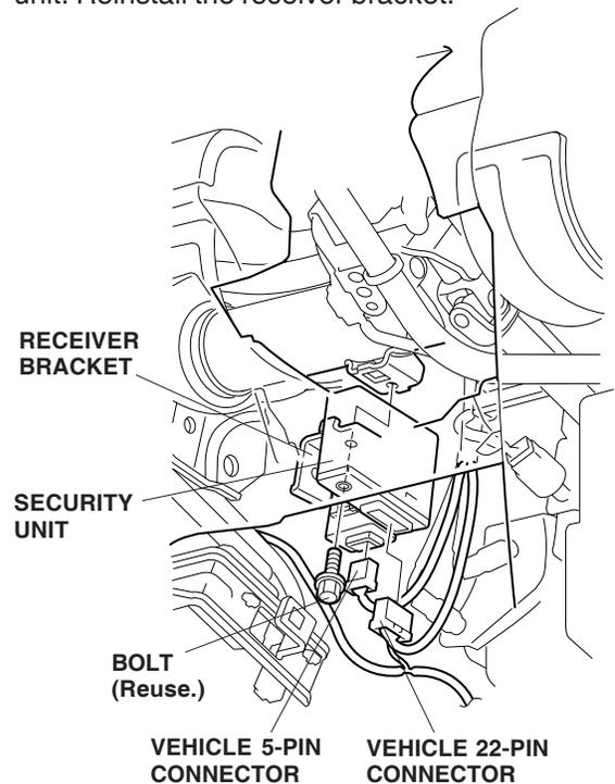
25. Reconnect the vehicle 5-pin connector to the keyless unit.
