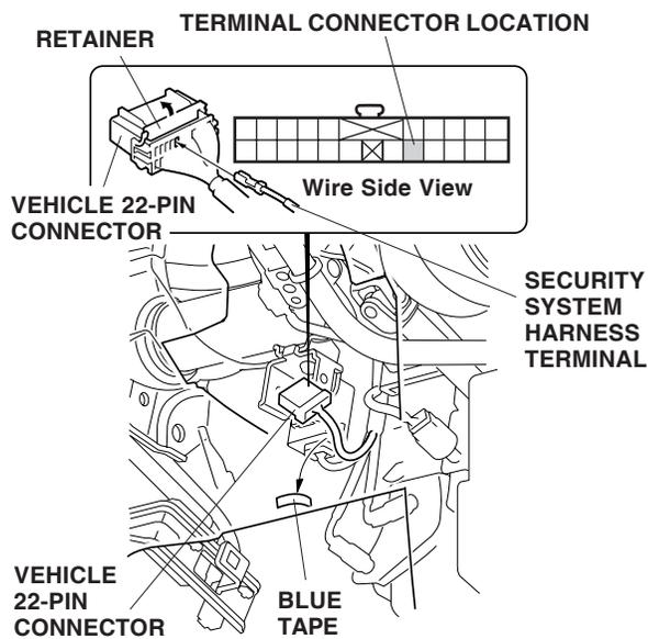
20. Push the security system harness terminal into the appropriate vehicle 22-pin connector terminal, then reinstall the retainer.
