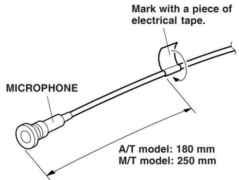
17. Route the microphone jack down through the hole in the shift lever cover, and seat the microphone.
