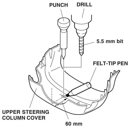
11. While wearing eye protection, lightly center-punch the mark, and drill a 5.5 mm hole through the upper steering column cover. Remove all burrs.
