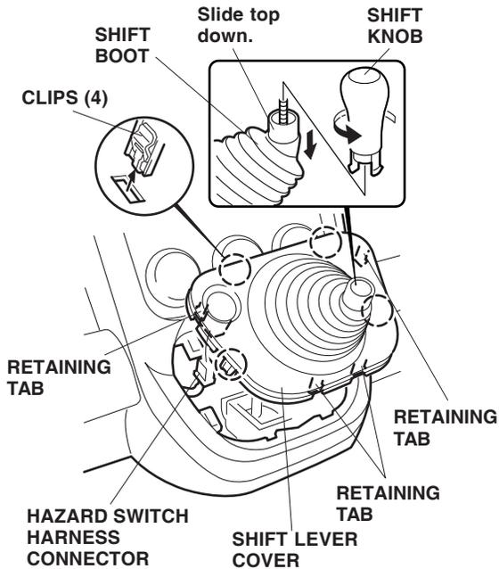
9. **On M/T model:** Reach through the shift boot, pull up the shift lever cover to release the four retaining tabs and four clips, and unplug the hazard switch harness connector.
