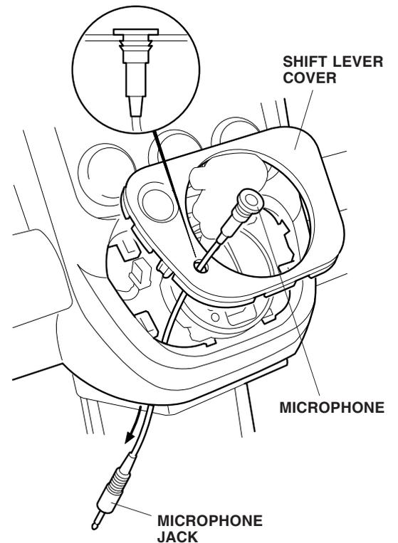
18. Reconnect the hazard switch harness connector, and reinstall the shift lever cover.
