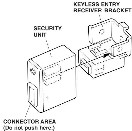
24. Plug the vehicle 22-pin connector into the security unit. Reinstall the receiver bracket.
