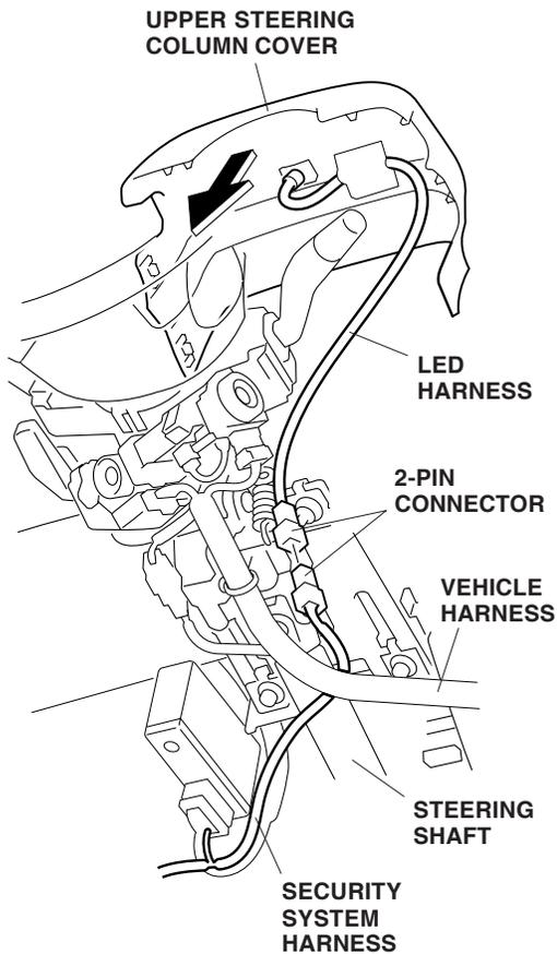
27. Route the security system harness 2-pin connector under the steering shaft, and connect it to the LED harness 2-pin connector.
