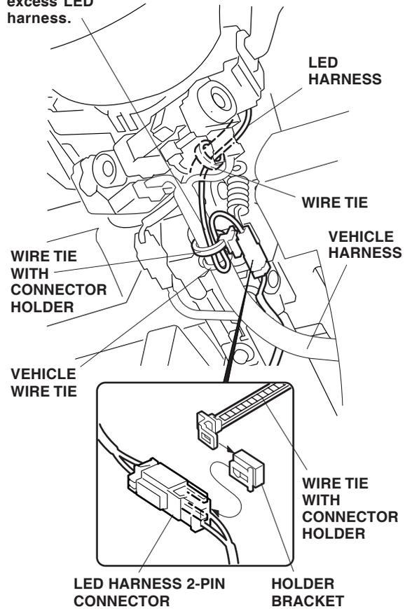
29. Secure the LED harness to the vehicle harness with one additional wire tie.
