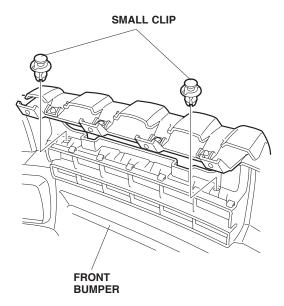
25. Reinstall the front bumper, check that clips and retaining tabs are installed securely.
