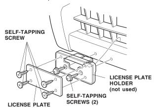
2. Remove the license plate holder (two screws).
