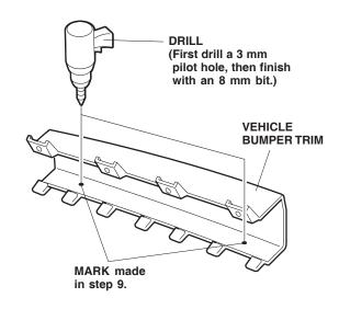
12. Using a felt-tip pen and a tape measure, mark the inside of vehicle bumper trim at the two locations shown.
