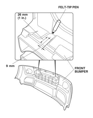
7. Lightly center punch the mark made in step 6, then while wearing eye protection, drill a 3 mm pilot hole and finish with a 8 mm drill bit. Remove any burrs from the holes.
