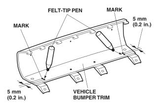
13. Inside the bumper trim, locate the five additional marks, and the two marks made in step 12. While wearing eye protection, drill a 3 mm pilot hole and finish with a 10 mm drill bit at each of the 7 marks. Remove any burrs from the holes with a file.
