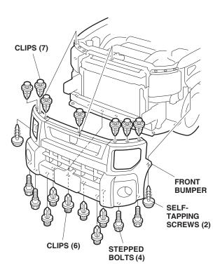
Starting at the end, pry up on the seven retaining tabs and remove the front bumper trim. Remove one clip at a time. Take care not to damage the retaining tabs.
