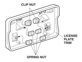
17. Align the license trim with the front bumper trim, and install the four self-tapping screws.
