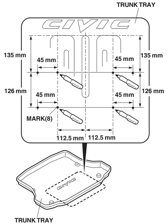
3. Using a pushpin, pierce at the eight marks you made on the trunk tray in the step 2. Drill the trunk tray at the pierced points using an electric drill motor with 5 mm bit. Remove the burrs from the edge of the holes.
