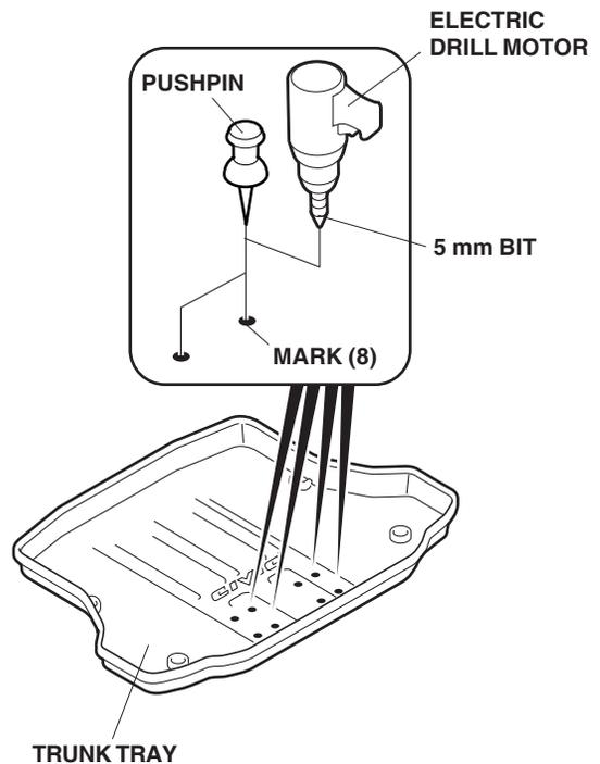
4. Using a utility knife, cut the trunk tray straight in the part between each of a pair of the holes you just drilled as shown.
