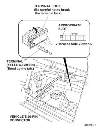
Carefully push the wire terminal (yellow/green) of the antenna sub harness into the appropriate slot of the vehicle 20-pin connector. Reattach the terminal lock.
