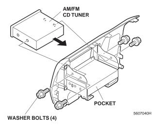
Fasten the two bolts on the right audio bracket you loosened in step 10, and reinstall the air duct. 20. Plug the vehicle 20-pin connector and antenna jack into the rear of the AM/FM CD tuner.
