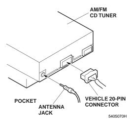
21. Connect the vehicle connectors to the center panel, and reinstall the center panel.
