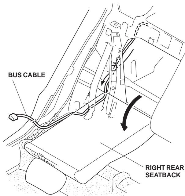
21. Return the right rear seatback, then remove the clip securing the floor carpet. Turn over the floor carpet.
