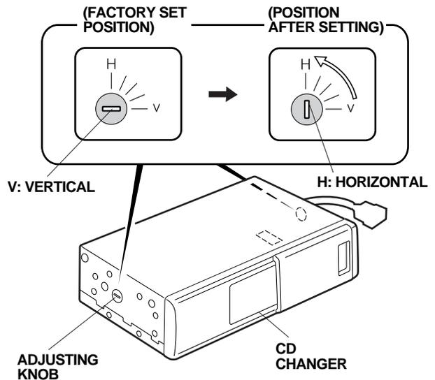
33. The adjustment knobs have been set to the vertical (V) position before shipping the CD changer from the factory. Move the adjustment knobs to the horizontal (H) position using a small flat-tip screwdriver.
