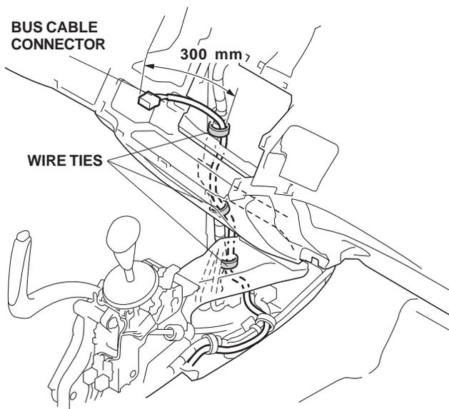
26. Secure the BUS cable to the vehicle harness with five wire ties.
