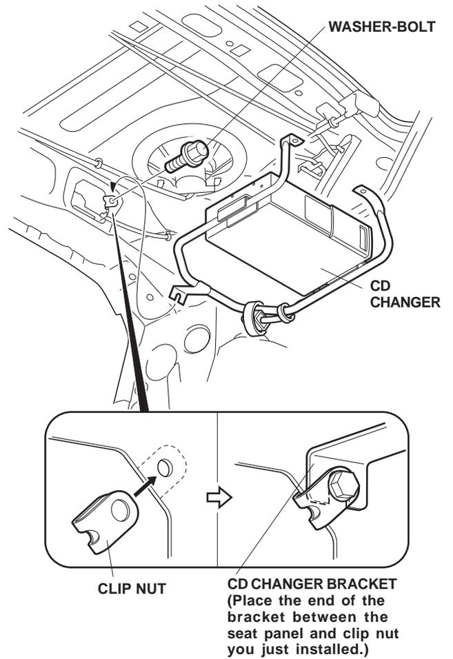
39. Slide the two clip nuts onto the CD changer brackets and parcel shelf through the holes in the parcel shelf, and align their holes as shown. Install the two washer-bolts, and tighten them securely.
