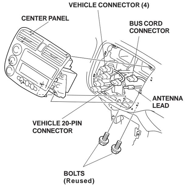
44. Check that all wire harnesses are routed properly and that all connectors are plugged in.
