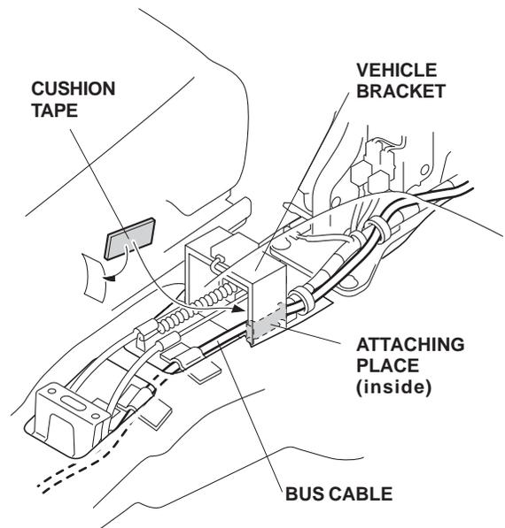
28. Turn over the floor carpet, and attach the BUS cable to the floor panel with the two cushion tapes in the areas shown.
