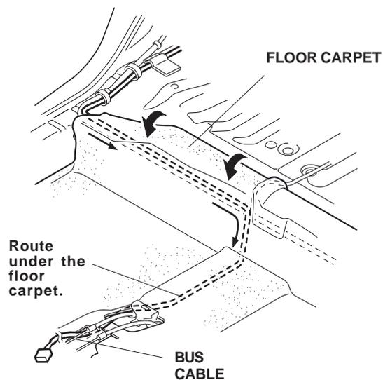
23. Route the BUS cable forward to the right front console frame along the vehicle harness.
