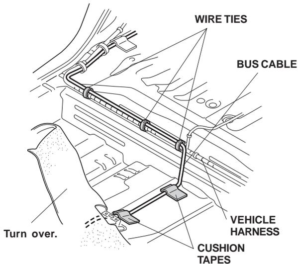
30. Secure the BUS cable to the vehicle harness with the two wire ties in the areas shown.
