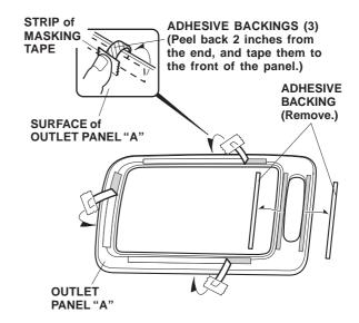
8. Attach the strip of masking tape to the end of each shaded adhesive backing. Peel back 2 in. (5 to 6 cm) of the adhesive backings, and fold them over as shown. Temporarily attach the strips of masking tape to the outside of the outlet panel "A." Remove all remaining adhesive backings from the outlet panel "A."
