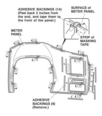
Position the meter panel on the existing meter panel. While holding pressure on the meter panel, carefully remove the adhesive backings from the meter panel. Hold the meter panel firmly against the existing meter panel with the palm of your hand, particularly at the edges.
