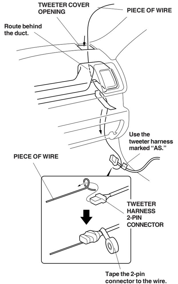
21. Pull the right tweeter 2-pin connector up from the floor to the tweeter cover opening.
