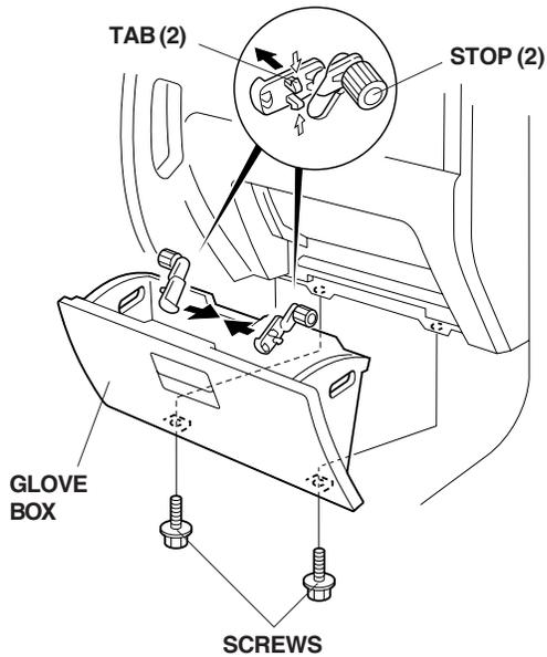
5. Remove the two screws from the bottom of the glove box, and remove the glove box.
