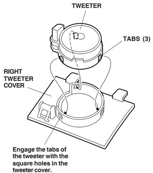
25. Plug the right tweeter harness 2-pin connector into the 2-pin connector of the tweeter, then reinstall the tweeter cover.
