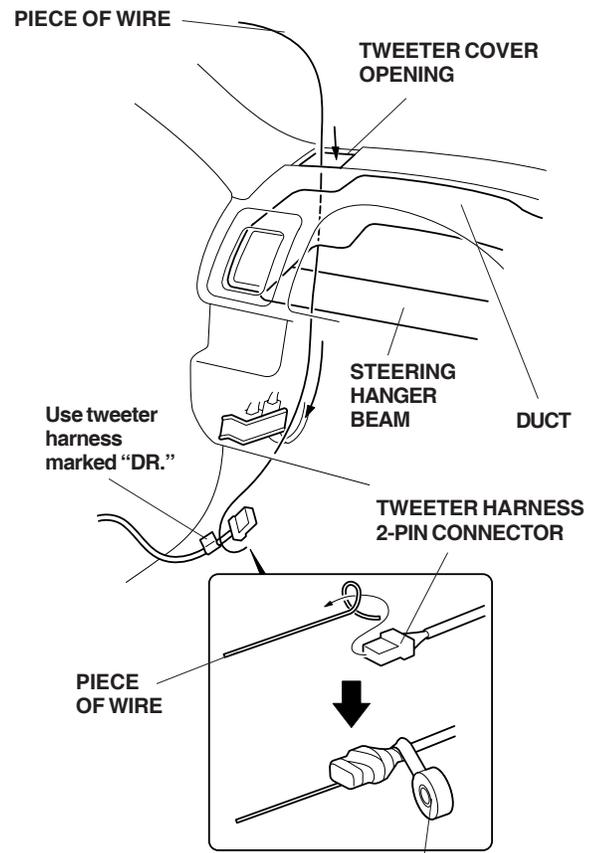
Tape the 2-pin connector to the wire.
