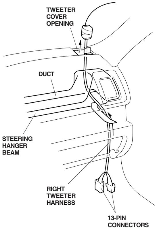
22. Remove the wire from the 2-pin connector. To prevent the tweeter harness from falling, tape it to the dashboard.
