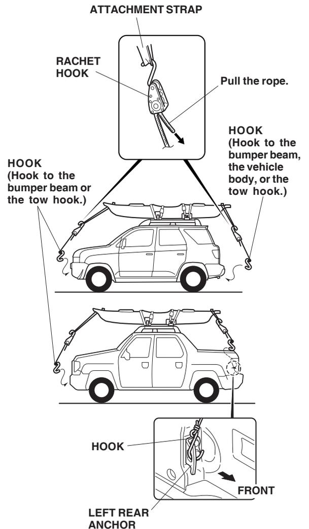
13. To loosen the rope, push up on the ratchet strap lever, then loosen the rope by pulling on the other end of the rope.
