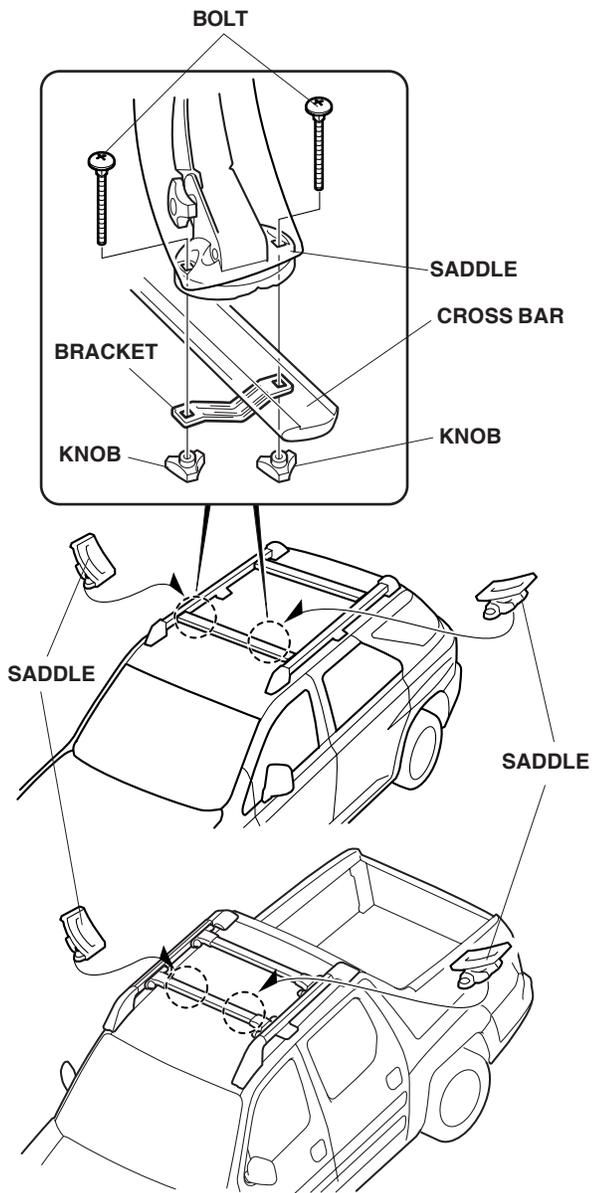
2. Position the two hydro-glide assemblies on the rear crossbar, and loosely install the hydro-glide assemblies using one bracket, two bolts, and two knobs for each assembly. The distance between the two assemblies should be the same width as the kayak.
