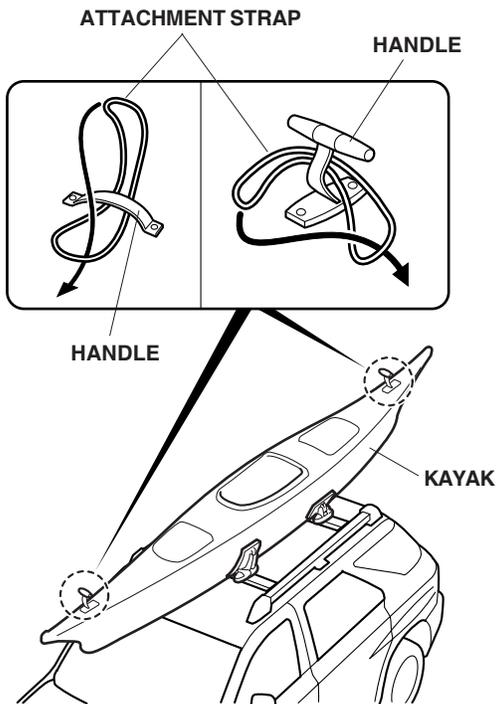
12. Attach one ratchet hook to the front attachment strap and one ratchet hook to the rear attachment strap. Hook the other end of the ratchet strap to the front bumper beam or to the tow hook. Hook the other end of the rear ratchet strap to the rear bumper beam, vehicle body, or to the tow hook. Secure the kayak to the vehicle by pulling the rope through the ratchet hooks.
