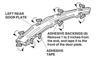
33. Align the edge of the left rear door plate with the edge of the left rear door.
