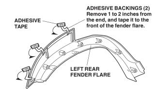
29. Position the left rear fender flare against the vehicle and secure the six clips into the holes of the body panel. Confirm that the edge of the left rear fender flare is aligned with the edge of the left rear fender.
