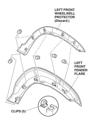
7. If equipped without a front splash guard, install the left front fenderwell cover to the left front fender flare using one clip from the kit.
