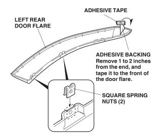
37. On the inside of the left rear door flare, remove 1 to 2 inches from the adhesive backing. Fold the end back, and tape it to the front of the door flare.
