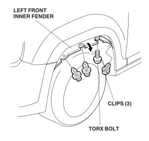
3. Remove the two self-tapping screws that fasten the left front wheelwell protector. Remove the five clips by squeezing the clip, and pulling the protector out toward you, then remove the wheelwell protector. Take care not to damage the clips.
