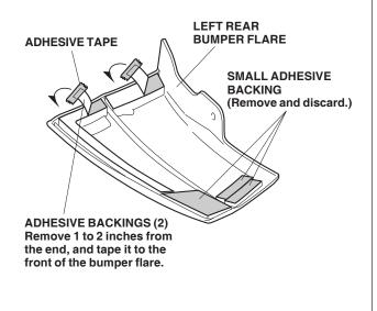
22. Position the edge of the left rear bumper flare with the upper edge of the rear bumper and place the flare onto the rear bumper. Install the left rear bumper flare with the self-tapping screw removed in step 19. Do not tighten the self-tapping screw yet.
