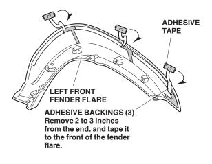
10. Position the left front fender flare against the vehicle and engage the five clips into the holes of the body panel. Confirm that the end of the left front fender flare is aligned with the end of the left front fender.
