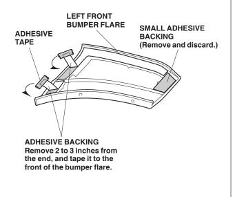
15. Position the left front bumper flare on the front bumper and install the two 5 x 20 mm self-tapping screws (from the kit) through the front bumper. Do not tighten the self-tapping screws yet.
