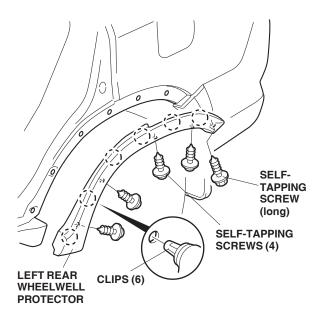
26. Remove the six clips from the left rear wheelwell protector, and transfer the clips to the left rear fender flare.
