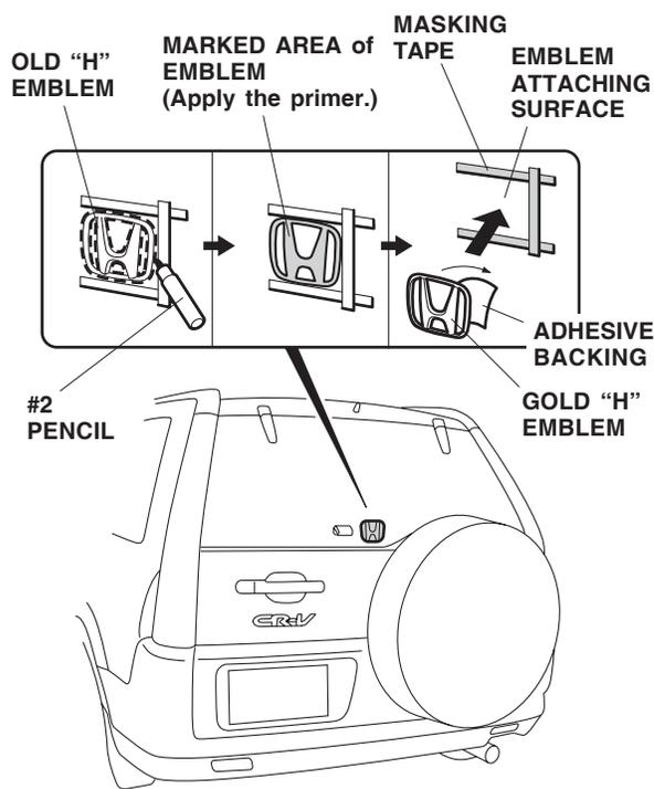
16. Wipe up any excess primer between the emblem using isopropyl alcohol.
