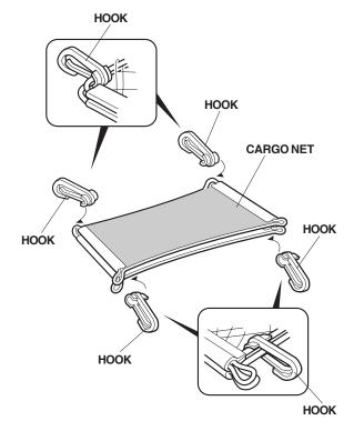
2. Attach the hooks to the anchors in the trunk. The cargo net can be installed in two different positions.
