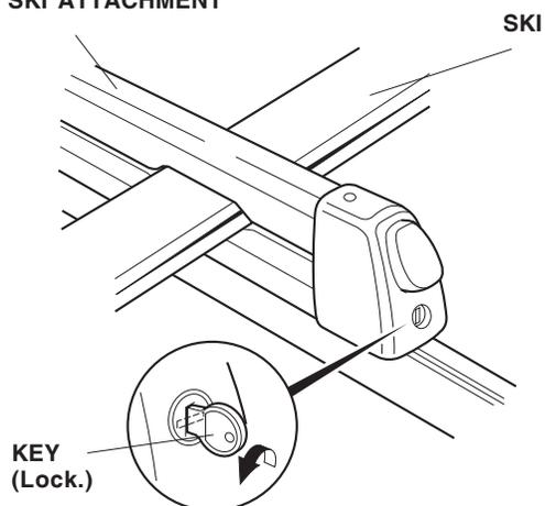
5. With the ski attached, rock the attachment in all directions to make sure it is installed securely. Adjust as necessary.
