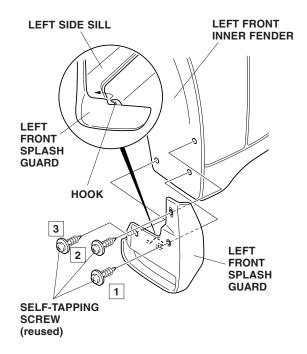
Turn the steering wheel all the way clockwise, and repeat steps 2 and 3 install the right front splash guard.
