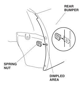
Position the left rear splash guard on the rear bumper and left rear inner fender, and install one self-tapping screw (short), one self-tapping screw (long) and one self-tapping screw removed in step 5. Tighten the three self-tapping screws in the order shown.
