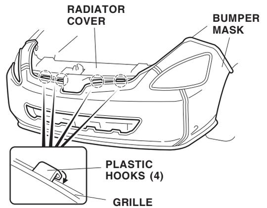
15. Hook the two elastic straps to the inside top edge of the grille opening, and attach the four plastic hooks to the bottom inside edge of the grille opening.
