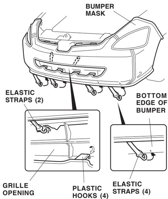
16. Hook the four remaining elastic straps to the bottom edge of the bumper.
