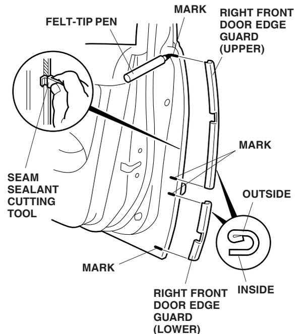
4. Position the cutting edge of the seam sealant cutting tool against the door edge, and trim the seam sealant from mark to mark, top and bottom.
