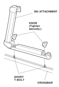
6. Repeat steps 4 thru 6 to install a ski attachment onto the rear crossbar.
