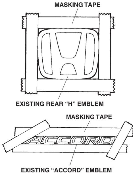
8. Remove the “H” and “ACCORD” emblems from the body by moving the string back and forth, and working it between the emblems and the body.
