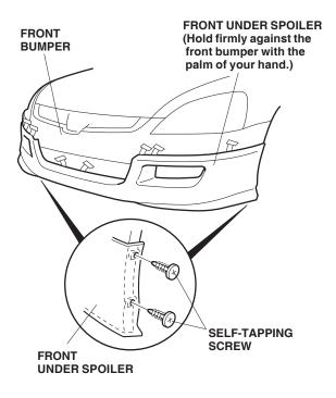
the sides, hold light pressure on the front under spoiler, and carefully remove the adhesive backings from the front under spoiler. Using the palm of your hand, hold the front bumper spoiler firmly against the front bumper for 30 seconds.
