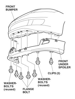
against the front bumper, install the two selftapping screws on each side. Do not tighten the self-tapping screws yet.
