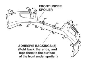
the front bumper where the front under spoiler will attach.
