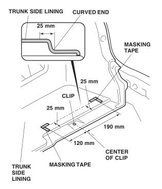
6. While wearing eye protection, drill 5 mm holes through the right side trunk lining and rear floor panel inside the right angles made by the masking tape. First drill with a 3 mm drill bit, and finish with a 5 mm drill bit.
