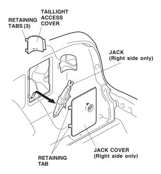
5. Measure the right side trunk lining and mark the measurements with masking tape in the areas shown.
