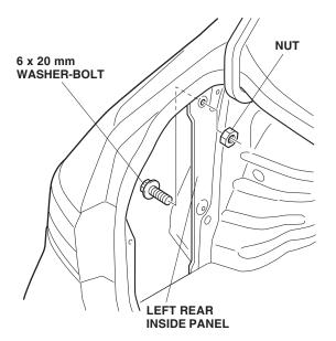
Using a white paint pen, apply white paint to the end of the washer-bolt.
