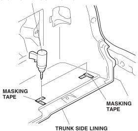
7. Repeat steps 5 and 6 to mark and drill holes in the left side trunk lining and rear floor panel.
