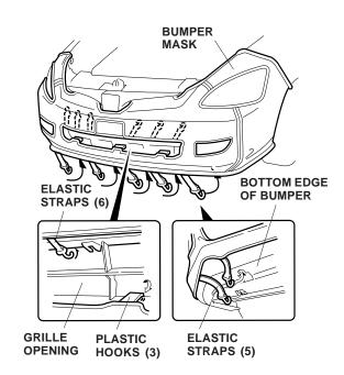
15. Attach the five remaining elastic straps to the bottom edge of the bumper.
