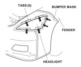
13. Attach the six plastic hooks to the top of the front bumper.
