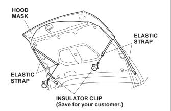
3. Fit the corners of the hood section around the hood, and adjust the mask so it fits smoothly over the edges. Attach the four elastic straps to the holes in the hood.
