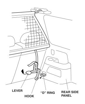
7. Adjust the length of the straps as needed. Lower the handle and snap the lever closed against the hook.
