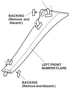
6. Position the left front bumper flare on the front bumper and install the three self-tapping screws (from the kit) through the front bumper. Reinstall the bumper bolt you removed in step 1, but do not tighten the self-tapping screws or the bolt yet.
