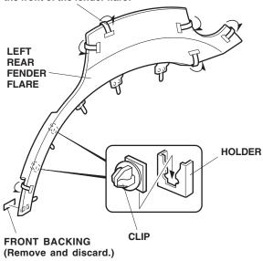
23. Slide one clip into each holder on the rear fender flare.
