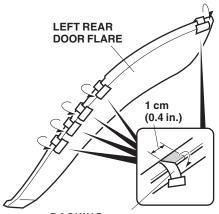
BACKING Remove 1 cm (0.4 in.) from the end, and tape it to the front of the rear door flare.
