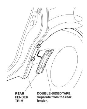
20. Remove and discard the two clips from the rear fender.
