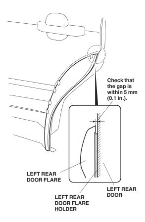
44. If the gap between the top edge of the left rear door flare and the left rear door is more than 5 mm (0.1 mm), repeat steps 41 through 43 to reinstall the left rear door flare.
