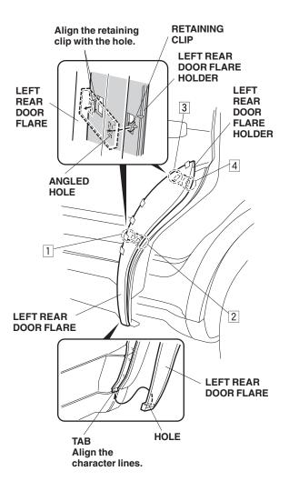
43. Check that the gap between the top edge of the left rear door flare and the left rear door is within 5 mm (0.1 in.).
