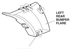
BACKING Remove 3 to 5 cm (1 to 2 in.) from the end, and tape it to the front of the fender flare.
