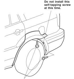
30. Reinstall the molding over the rear fender and fender flange.
