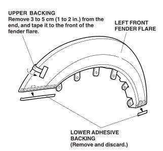
12. Align the ends of the front fender flare with the front end of the front fender, and bend the mounting tabs around the fender flange.
