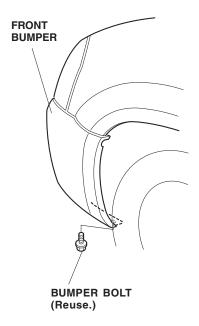
Align the ends of the front bumper flare with the front end of the front bumper, and bend the mounting tabs around the fender flange. Using a felt-tip pen, mark the edge of the front bumper through the three holes in the bumper flare. Remove the front bumper flare.
