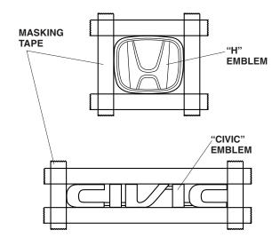
7. Remove the original rear emblems by cutting the outer edges with a piece of string. Note the locations of the locating pins of the emblems.
