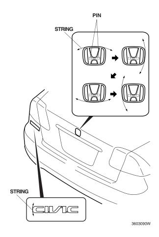
8. Remove the two clips from the trunk lid. Be careful not to damage the body.
