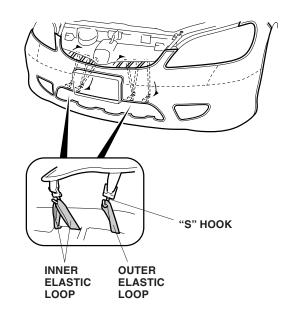
13. Attach the four plastic hooks to the bottom edges of the bumper grille.
