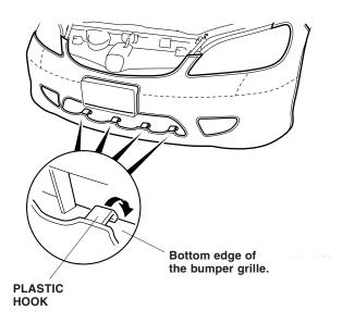
14. Route the elastic cord through the eight loops on the bottom of the mask. Attach one "S" hook to the bottom edge of the bumper on one side. Stretch out the cord after routing it through each loop then attach the other "S" hook to the bottom edge of the bumper on the other side. Attach the hooks on the corners of the mask to the bottom edge of the bumper on both sides.
