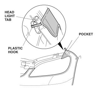
8. Pull the mask back toward the wheelwell, smooth out any wrinkles, and then snap the mask onto the snap-screw. Repeat on the other side.
