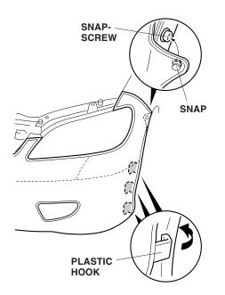
9. On both sides of the vehicle, attach the three plastic clips to the fenderwell.
