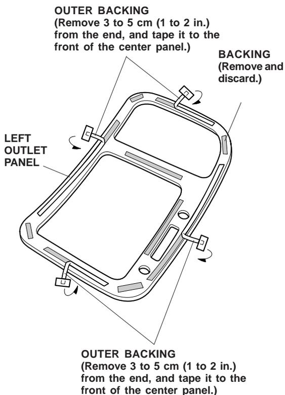
9. Position the left outlet panel on the outlet in the position noted in step 7. As you apply pressure to the outlet panel, slowly and carefully remove the backing from the outlet panel. Hold the shift panel firmly against the existing shift panel with the palm of your hand for 30 seconds.
