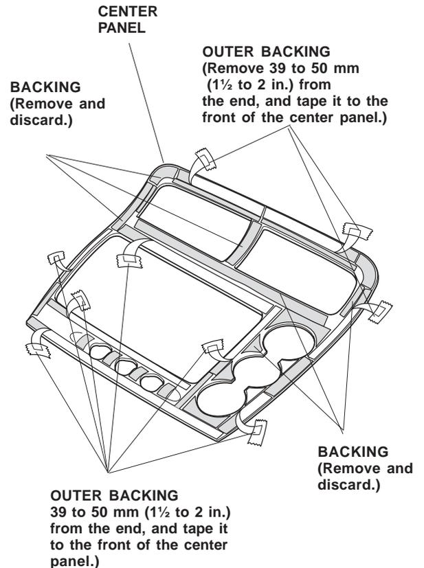
3. Angle the center air outlet louvers down. Position the center panel on the existing center panel in the position noted in step 1. As you apply light pressure to the center panel, slowly and carefully remove the backing from the center panel. Hold the new center panel firmly against the existing center panel with the palm of your hand for 30 seconds, particularly at the edges.
