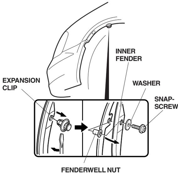
5. Pull the inner fender away, and press one fenderwell nut (supplied) into the hole in the fender flange.
