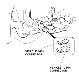
32. Slide the vehicle 4-pin connector you just removed onto the 10-pin connector of the main harness, then reconnect the harness.
