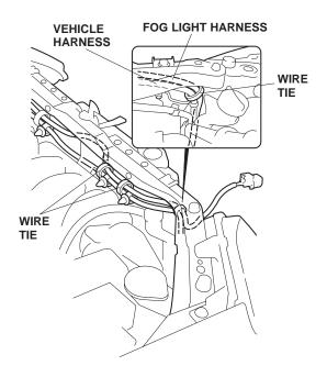
43. Secure the fog light harness to the vehicle harness with two wire ties.
