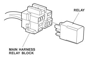
24. Slide the relay block of the main harness onto the vehicle bracket.
