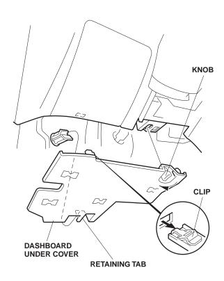
20. Remove the two self-tapping screws that secure the top of the pocket, and remove the pocket by removing the two clips and one retaining tab.
