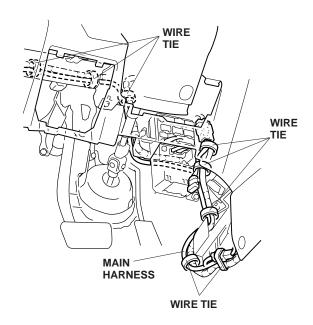
35. At the left (driver's side) kick panel, secure the main harness to the vehicle harness with three wire ties in the areas shown.
