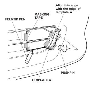
7. Remove templates A, B and C. While wearing eye protection, drill a 10 mm hole through each of the three marks. First drill with a 3 mm bit, then finish with a 10 mm bit.
