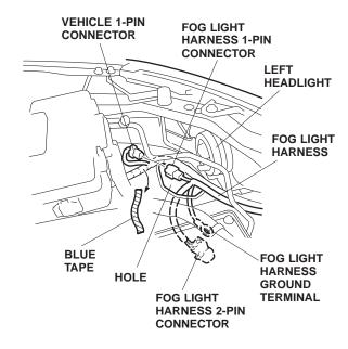
39. Route the other 2-pin connector of the fog light harness to the right, along the vehicle harness, then secure the harness with three wire ties in the areas shown.
