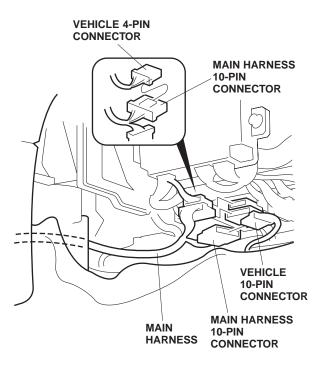
33. On the passenger's side, secure the main harness to the vehicle harness with three wire ties in the areas shown.
