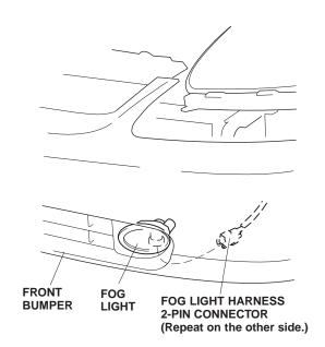
47. Plug in the side marker lights, and reinstall the front bumper. Check that all clips and retaining tabs are installed securely.
