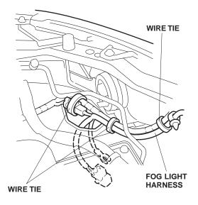
40. Attach a piece of wire to the 2-pin connector of the fog light harness. Using the wire, route the connector through the bulkhead, around the latch and back through the bulkhead, then along the vehicle harness, toward the right headlight.
