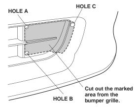
Inside the front bumper, temporarily slide the two spring nuts onto the bumper grille as indicated by the guide lines. Using a pushpin, mark the bumper grille at each of the two holes in the spring nuts. Remove the spring nuts.
