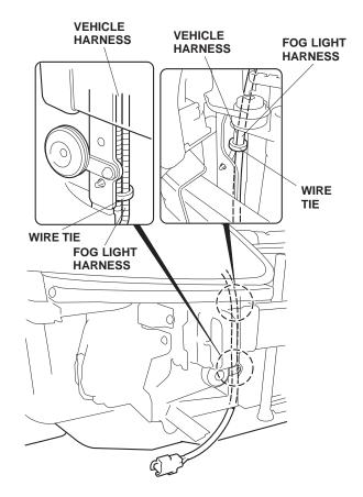
44. Loosen the central ground bolt, and secure the fog light harness ground terminal with this ground bolt.
