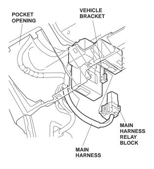
25. Pull the 5-pin connector of the main harness out through the switch hole, then plug it into the switch. Install the switch in the switch hole.
