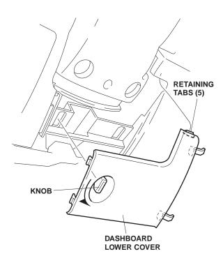
19. Remove the driver's dashboard under cover. Turn the knob clockwise, and release the clip and one retaining tab.
