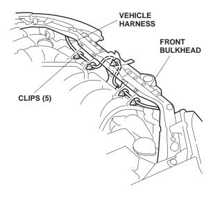
38. Behind the left headlight, locate the 1-pin connector blue-taped to the vehicle harness, and remove the blue tape to free the connector.
