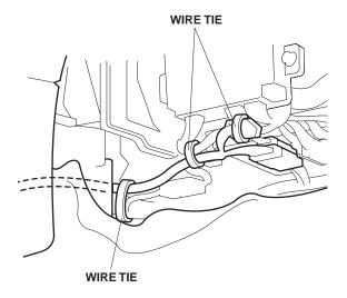
34. On the driver's side, secure the main harness to the vehicle harness with eight wire ties in the areas shown. This harness is near the brake pedal bracket, about 150 mm (6 in.) above the steering shaft.
