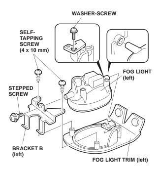
14. Install one stepped screw and one washer-screw to secure the fog light to bracket B and fog light trim.
