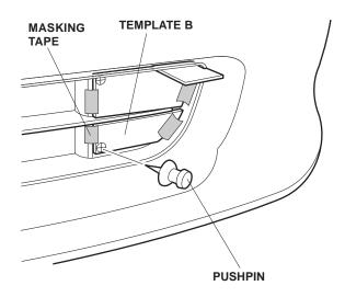
6. Cut out the template C, and tape it onto the front bumper by aligning the inner edge with the left edge of the bumper grille as shown. Using a pushpin, mark the bumper grille as indicated on the template. Using a felt-tip pen, mark the bumper grille along the outer edge of the template as shown.
