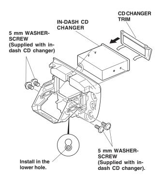
13. Bend the two bottom plates of the CD changer trim around the edge of the center panel.
