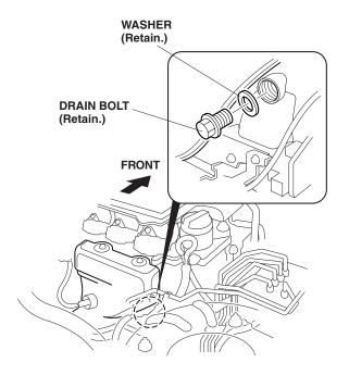
5. Install the new aluminium washer and the engine block heater into the bolt hole using a 24 mm socket and a torque wrench. Torque the engine block heater to 60 N·m (44 lb-ft).
