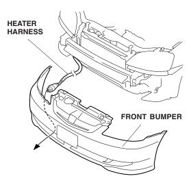
10. Continue routing the heater harness to the left, along the front bumper grille, and secure it to the bumper grille with four wire ties in the areas shown.
