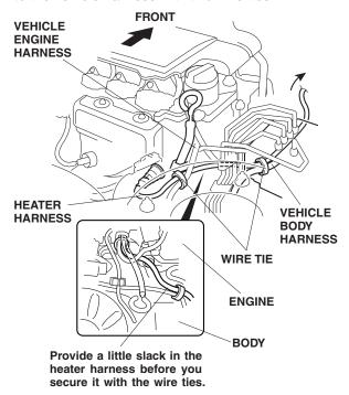
8. Route the heater harness connector out through the opening under the right headlight, and secure the harness to the vehicle harness hole in the right front bulkhead panel and lower cross member with the six wire ties as shown.
