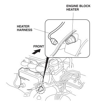
7. Route the heater harness along the vehicle engine harness and vehicle body harness, and secure it to the vehicle harness with two wire ties.
