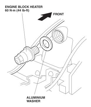
6. Plug the connector of the heater harness into the engine block heater.
