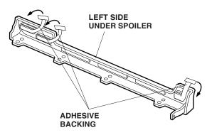
Position the four brackets B on the left side under spoiler, and secure each bracket with one screw.
