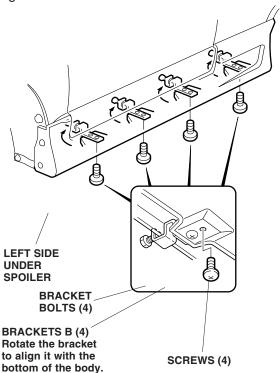
18. While holding light pressure on the left side under spoiler, carefully and slowly remove the adhesive backings. After installing, hold the spoiler firmly against the body with the palm of your hand for at least 30 seconds.
