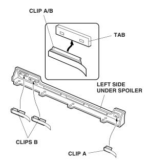
4. Position the left bracket A on the front end of the left side under spoiler and secure it with a clip.
