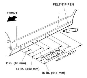
8. Open the door, align the template with the mark and mark the body at the six locations as indicated by the arrow on the template.
