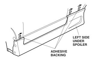
19. Turn the steering wheel all the way clockwise, and repeat steps 1 through 18 to install the right side under spoiler.
