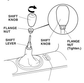
11. Install the shift knob on the shift lever until it is tight, then place it in the correct location, and tighten the flange securely.
