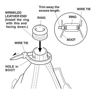
6. Secure the boot to the ring with the wire tie as shown.
