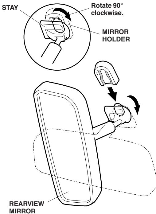
6. Replace the mirror spring. Slide the day/night mirror stay onto the mirror holder, then turn the mirror stay counterclockwise as shown.
