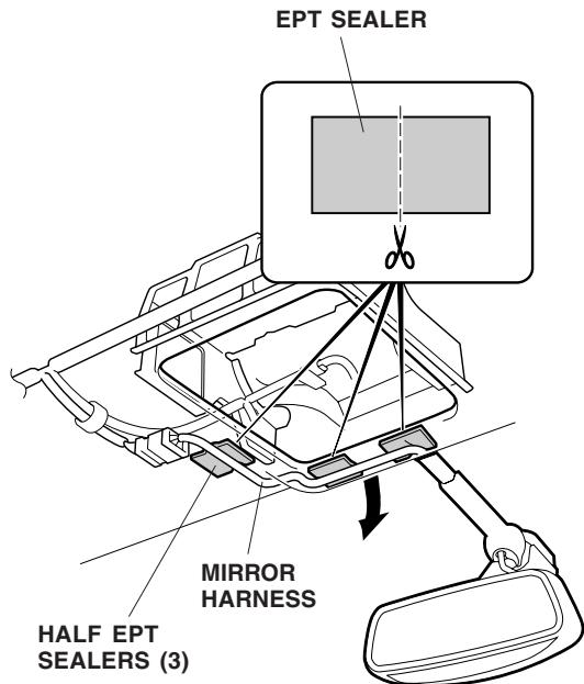
13. Using scissors, cut the two EPT sealers in half.
