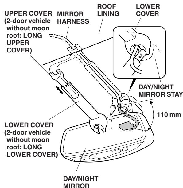
11. Remove the dummy connector from the vehicle harness 3-pin connector, then connect the vehicle harness 3-pin connector to the mirror harness 3-pin connector.
