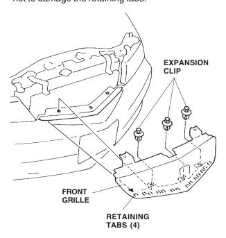
3. Inside the front grille, cut off the two pins, and remove the push nuts.
