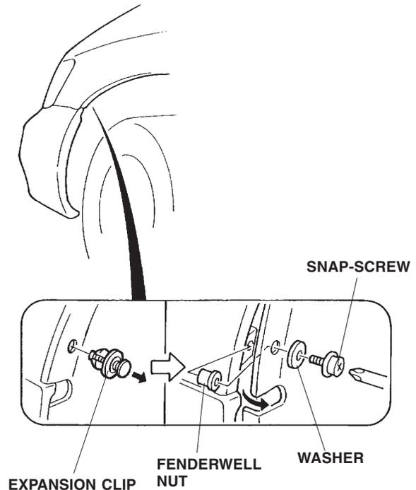
6. Pull out on the inner fender, and press one fenderwell nut into the hole in the fender flange.
